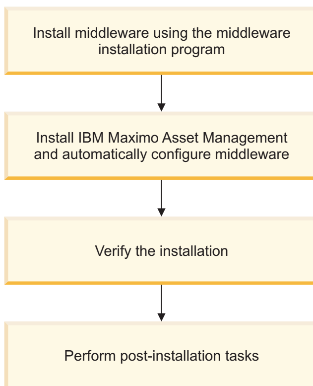
Figure 1. Deploying Maximo Asset Management using automatic middleware configuration
